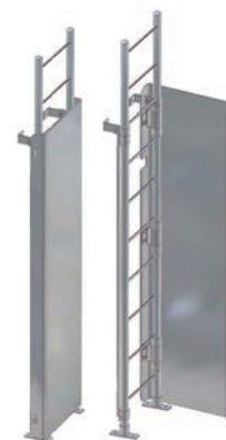
SL/LG LADDER GUARD The padlockable ladder guard designed to fit onto our SL ladders to prevent unauthorized use. LG2 - 2m long, LG25 - 2.5m long.
